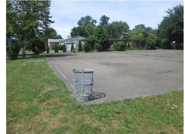
This play area contains two paved areas, a blacktop and a basketball court, which drain to the surrounding grass and roadway. The runoff from the basketball court primarily flows toward the northeast corner where a rain garden can be installed to capture, treat, and infiltrate stormwater. The blacktop can also be redone with pervious pavement to infiltrate runoff. A preliminary soil assessment suggests that the soils have suitable drainage characteristics for green infrastructure.
